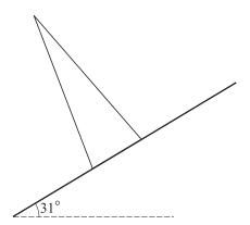
The cone is placed with its axis vertical on a rough horizontal plane. The plane is slowly tilted, and the cone remains in equilibrium until the angle of inclination of the plane reaches  $31^{\circ}$  (see diagram), when the cone topples.
