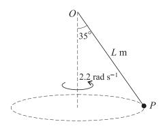
A particle P of mass  $m \log i$  is attached to one end of a light inextensible string of length L m. The other end of the string is attached to a fixed point O. The particle P moves with constant speed in a horizontal circle, with the string taut and inclined at 35° to the vertical. OP rotates with angular speed  $2.2 \, \text{rad s}^{-1}$  about the vertical axis through O (see diagram). Find
